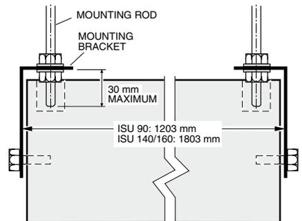
3. Thread on and tighten the lower washer and locknut sets (not supplied) to secure the left and right mounting brackets. **Note:** Mounting bracket flanges face inwards.
