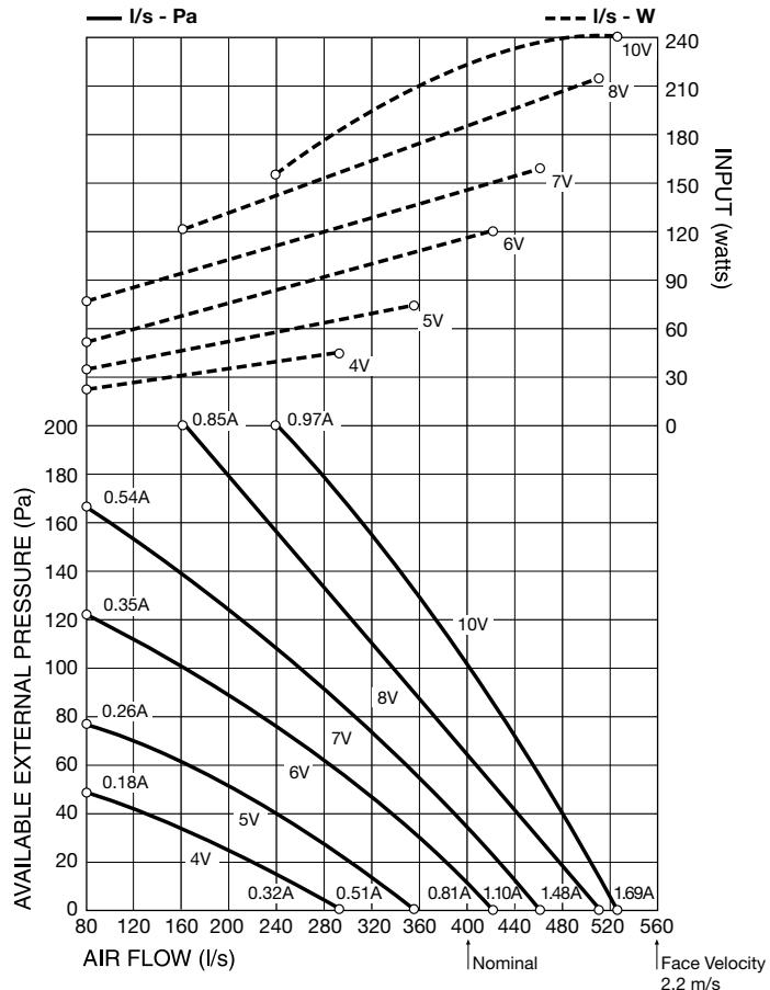
**Note:** Airflows are for dry coil. Reduce airflow by 10% in high moisture removal conditions.
