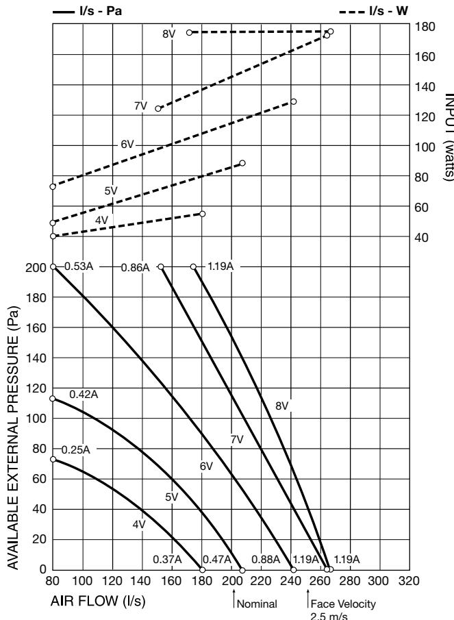
**Note:** Airflows are for dry coil. Reduce airflow by 10% in high moisture removal conditions.
