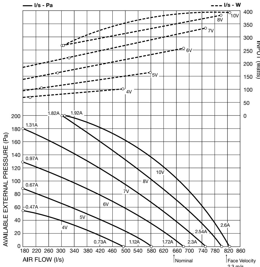
**Note:** Airflows are for dry coil. Reduce airflow by 10% in high moisture removal conditions.
