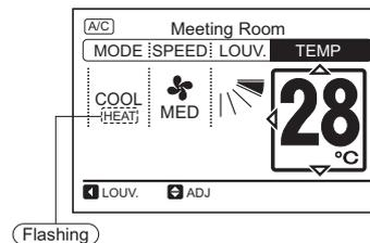
Indication when "COOL" operation is set by the remote control switch at the outdoor unit "HEAT" operation.
