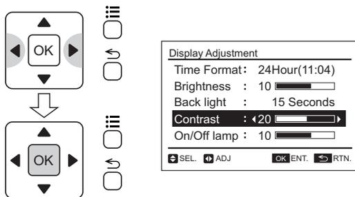
(5) Select “Yes” by pressing “◀” or “▶” and press “OK”. The setting will be confirmed and the screen will return to the normal mode.
