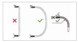
\* Never use a banding radius less than the minumum amount shown in the table. To prevent twisting and distortion, hose should be bent in the same plane as the motion of the boss to which the hose is connected.
