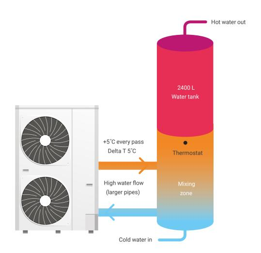
Multi-Pass system inefficient system design For example, a Multi-Pass system storage tank must contain sufficient volume to meet the entire peak usage period (in this example 2400 litres). Whilst the system will begin to reheat the water this hot water is not available until the entire tank reaches a usable temperature.
